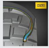
What is it? Casing reinforced with a spiral overlay of steel or aramid
