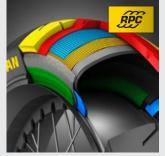
What is it? Front tyre carcass incorporating Rayon as ply material because of its thermodynamic properties, in order to meet specific performance requirements
