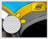
What is it? Front tyre carcass incorporating Rayon as ply material because of its thermodynamic properties
